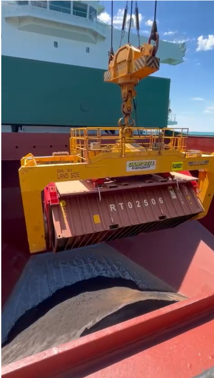
Caption: A rotainer of ilmenite being loaded onto a bulk carrier at the Port of Broome.
