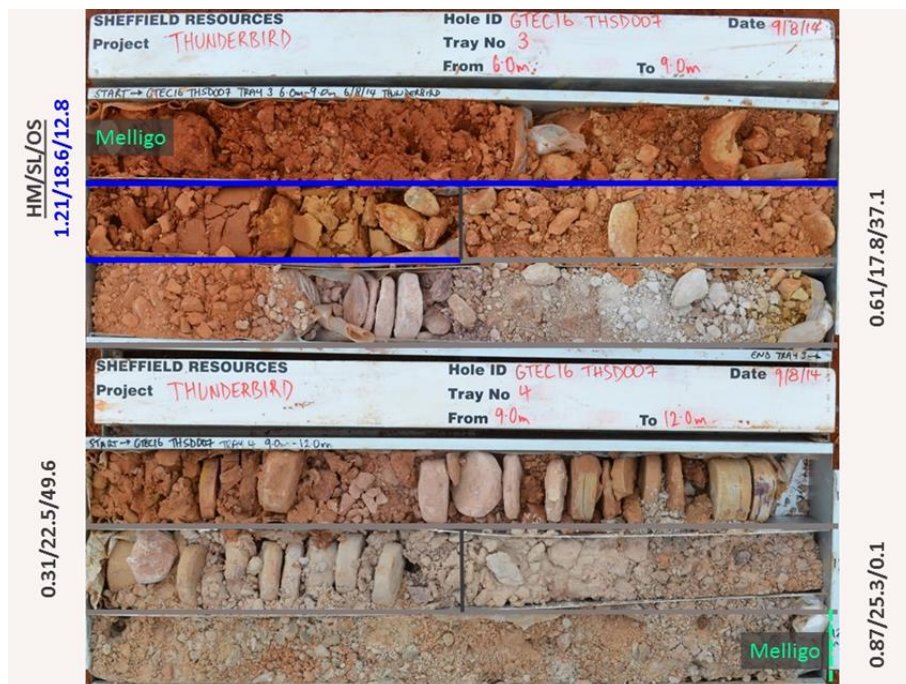
Figure 3: Upper portion of drillhole THSD007 noting Pindan Sands and Melligo Sandstone intersections.
